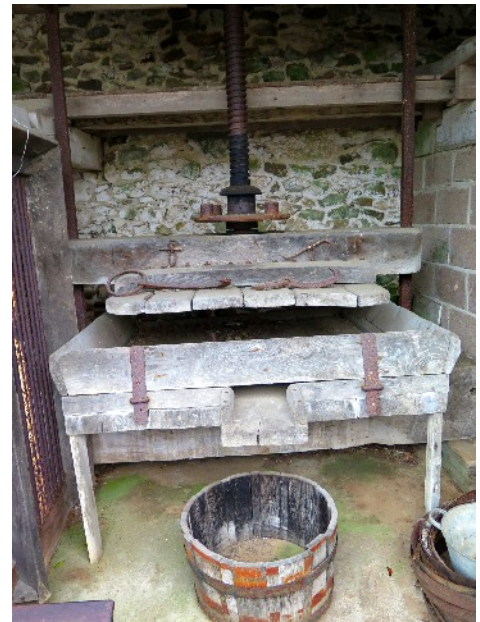
Mid 18 th century Cider Press - metal screw is mid 19 th century and originally it had 2 wooden screws
